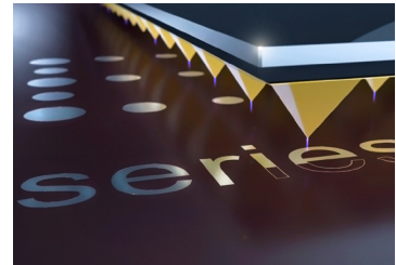
Massively parallel BPL tip array with millions of tips
